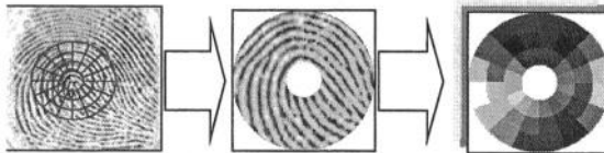
Fig. 3. The main steps of the fingerprintcode feature vector generation. A circle decomposed in a certain number of sectors is centered on the core of the fingerprint image. A set of Gabor filters is applied to such tessellated image. The standard deviation of the gray level values of each sector of the filtered image are computed, so generating the fingerprintcode feature vector [9].
